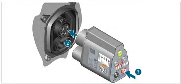
✓ You can now perform measurements in accordance with the guided fault finding.
